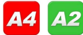
Generally - pick A4 grade if parts are used in any marine environment or, on land but close to the sea. A2 stainless is fine inland. However, there can be slight tarnishing over long periods of time compared with A4 stainless.
