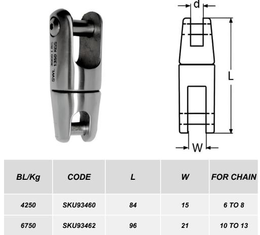
Notes : Dimensions are a guide and may vary slightly. Pls check with us for dimension critical applications. If Break (BL), Safe working load (SWL) or Working load limit (WLL) are shown: This is a guide only. (Do not use for lifting unless it is a certified lifting product)
