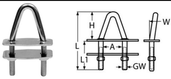
Strong U bolt with thick V section and 2 plates. With the two plates, it can be used to give a lashing point on the deck of the boat. The angled head makes side loading less likely, when Securing an item with rope. The top plate is fixed and welded.
