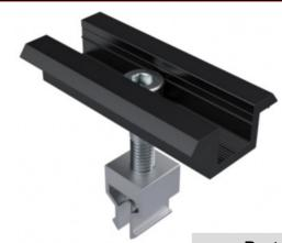
Adjustable clamps for solar panel depths of 30 to 40mm. Clip them into the rail and tighten. The clamp adjusts to the depth of the solar panel - anywhere between 30 & 40mm This pushes in to Steelgear Clip rails anywhere along the length of the rail. It is also compatible with the Schletter Eco and Solo rails
