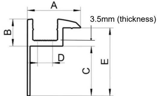
This clamp is designed for a DIN912 M8 socket cap head screw. Use dimension C + 3.5mm to help calculate the length of bolt for your project
