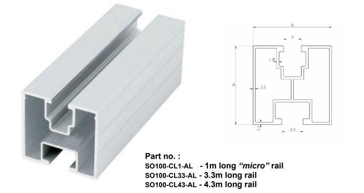
High strength mounting rail - 40x40 square mm. Uses Clip in in system for mounting clamps And uses M10 hammerhead or Hex head bolt for the roof hook fixing. This rail is also compatible With Schletter rapid clamps and fasteners
