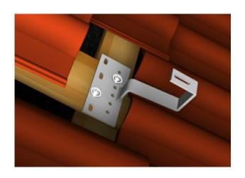
Woodscrew for securing solar roof hooks to wooden joists. M6x80 long. Hex head suitable for 10mm socket. Complete with EPDM rubber washer Use 2 per roof hook
